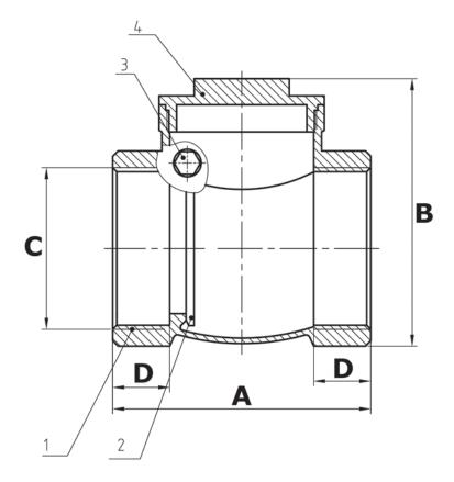
SPECIFICATIONS 125 SWP/300 W.O.G. THREADED CAP INTEGRAL BRASS SEAT THREADS CONFORM TO B1.20.1 RUBBER LINER NBR 75
